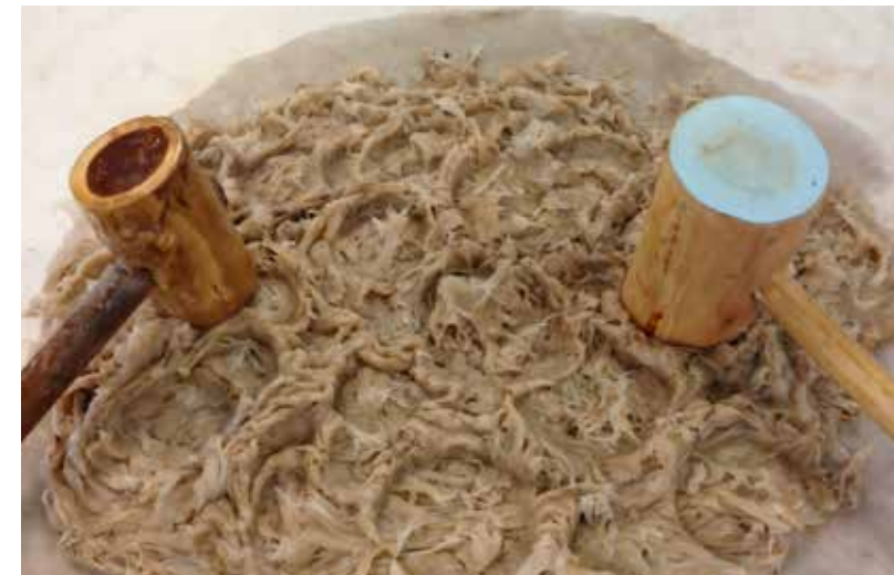
4. Beat fibers to correct length before coloring and adding to a vat of water.
